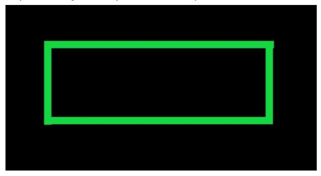
However, keep in mind that your camera may be looking at the target from an odd angle. This can drastically affect the aspect ratio of its contour. Be sure to test your settings from a variety of angles to ensure that you do not filter too aggressively and end up ignoring the vision target!
