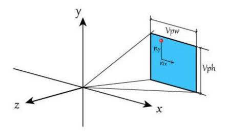
Given a distance of 1.0 unit and a known horizontal and vertical fov, we can compute the size of the view plane rectangle the following formulas:
